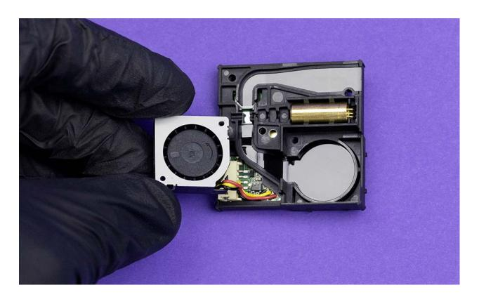
There is a small pocket underneath the fan that acts as its inlet. The air is then pulled up through the fan and exhausted out the other side.
