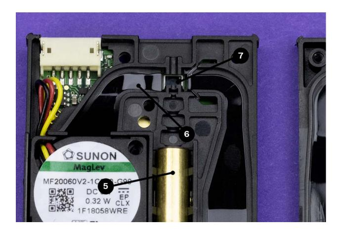
We can see these features in the Sensor. The laser (*Part 5*), the airflow path (*Part 6*), and the photosensor (*Part 7*).
